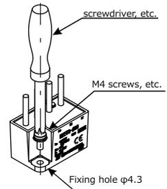
When installing, no separation distance from the ground conductor, etc. is required.
